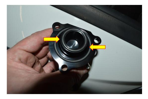
6. Take the Forge Motorsport valve and mount it into position where the OE valve was housed. Use the original T25 Torx fasteners to secure it in place.
