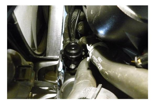
7. The next set of pictures are for illustration purposes - they may not be representative of your engine, but they are the clearest way to show you how to connect your solenoid to the atmospheric or recirculating valve you have fitted. Use the supplied silicone hose to do this, use a sharp knife or side cutters to cut the hose to length.
