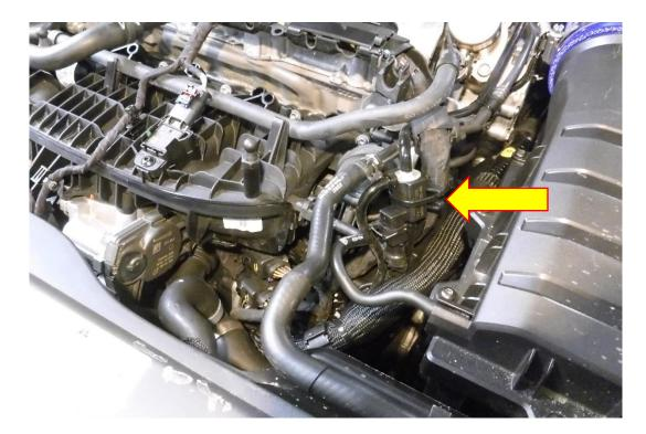
9. The vacuum source in the engine bay is next to where the solenoid has been fitted. Pull the vacuum pipe away from the plastic joiner.
