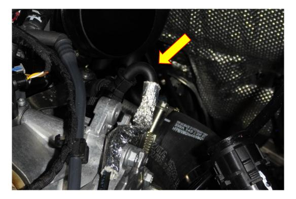
10. Using the supplied brass T piece and silicone pipe attach it to the vacuum pipe removed in the previous step just like it is in the picture below. Use the provided cable ties to secure the hose as shown with the arrows in the picture below.
