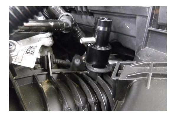
5. Attach the supplied silicone hose to the side pipe and run it to the back of the engine as illustrated below. Fit the OE Norma fitting back on and refit the engine cover.
