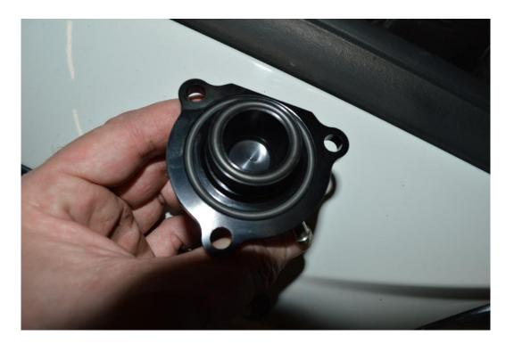
10. Fit the Forge valve to the turbo using the original fasteners and a T30 Torx drive.
