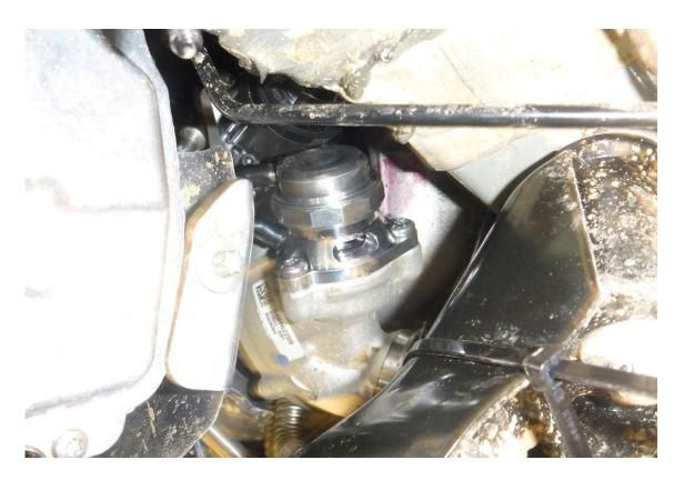
**11**. Fit the Forge wiring harness to the vehicle DV loom, you will hear a positive click when fully engaged.
