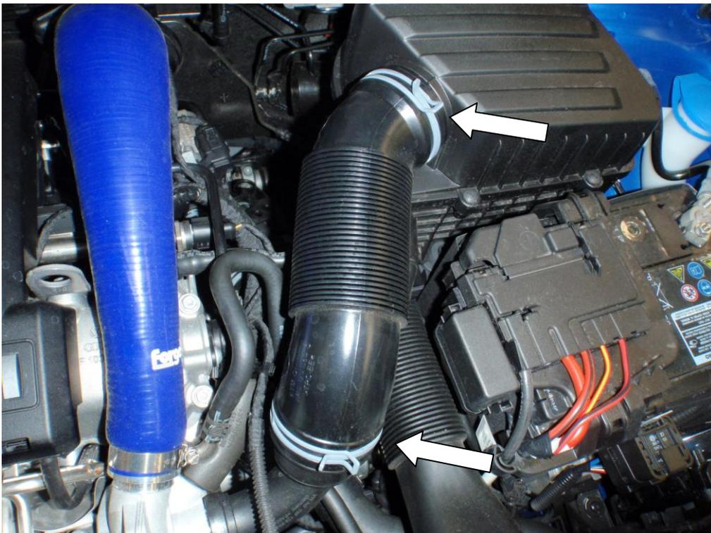
5. Undo the T25 screws holding the cold air feed and remove then undo the T30 torx screws on the turbo hosing holding the resonator pipe and remove.
