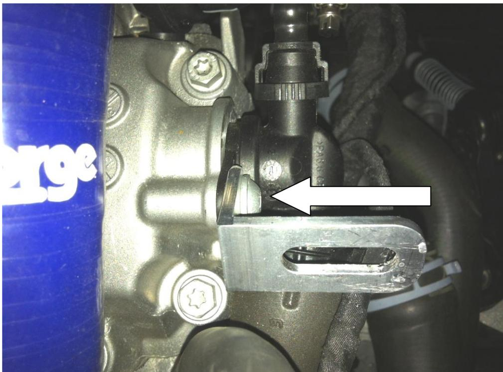
12. Secure the hose to the bracket using the P clip and supplied 5mm Allen head bolt.
