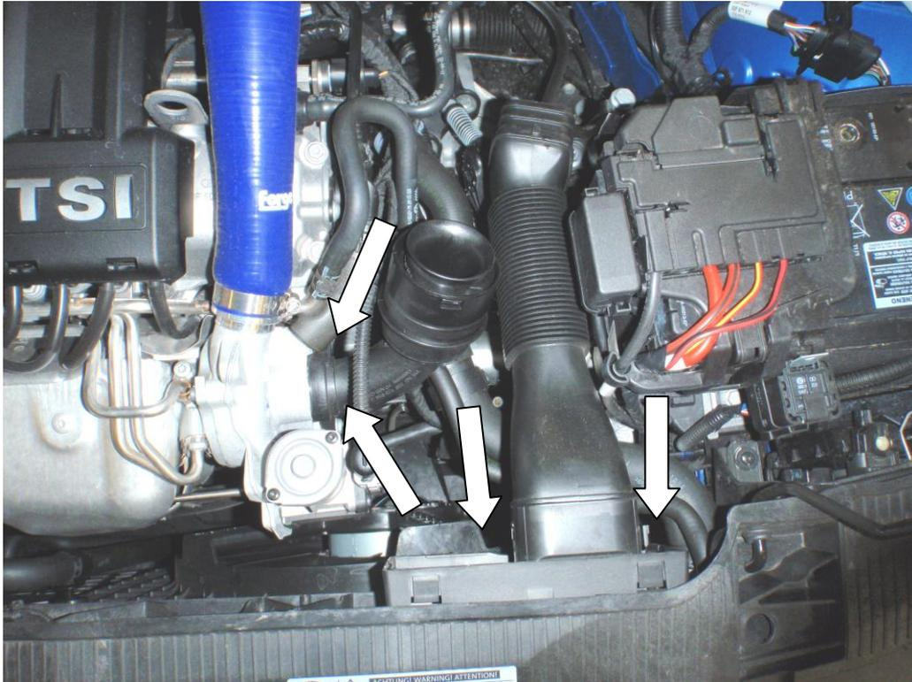
6. Connect the supplied turbo inlet connector using the supplied 5mm Allen head bolts.
