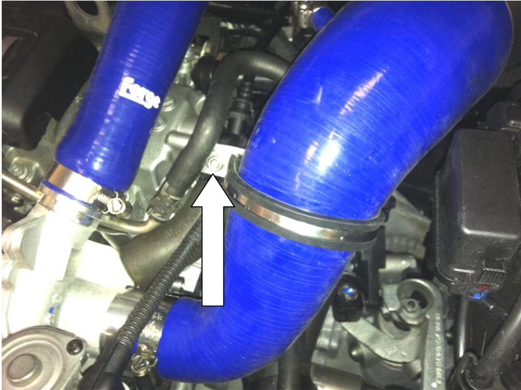
12 Check all hose clamps are tight also that all bolts are tight then road test vehicle.
