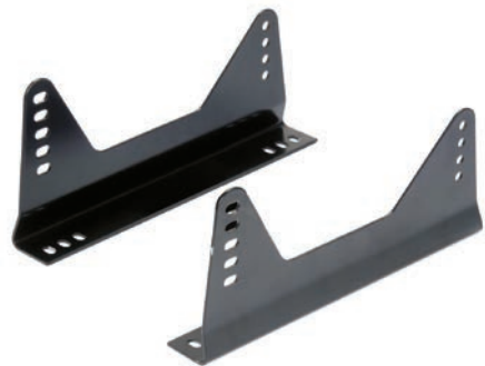
F1 Z200087 Steel brackets, th. 3mm, in compliance with FIA.
