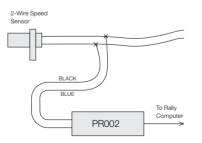
• The polarity of the connections does not matter.
